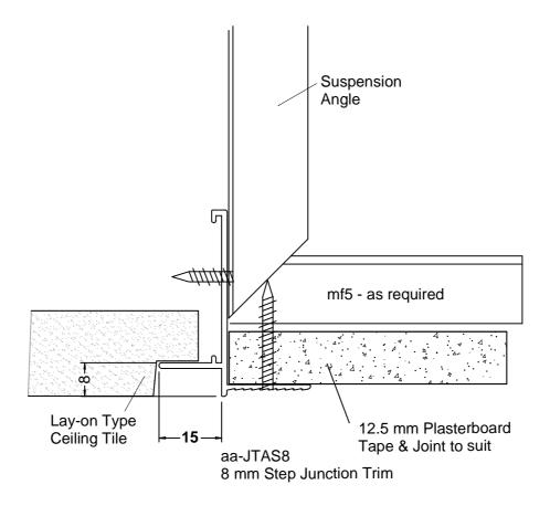
JTAS8 trim, used to create junction details between mineral fibre, g.r.g, or full module metal ceiling systems with an 8mm Tegular edge and adjacent areas of plasterboard. Manufactured from extruded aluminium, supplied in 3000mm lengths. Standard finish polyester powder coat to RAL9010, 20% gloss. Other finishes are available.
